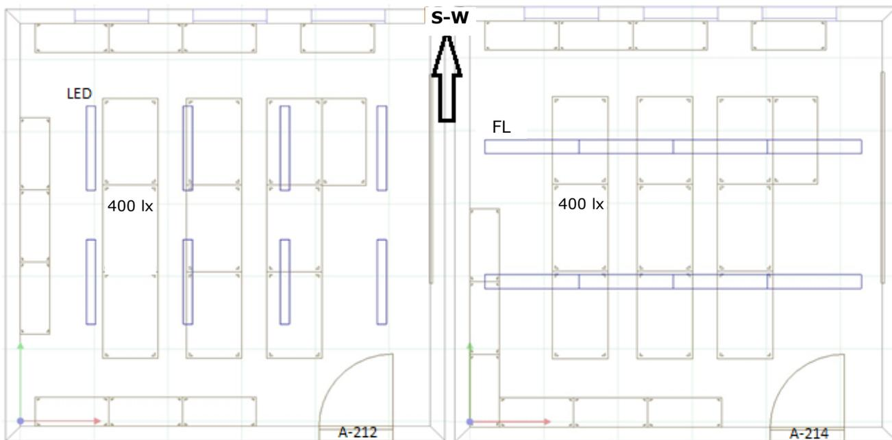
*Diagram 1 – Classroom plans with LED-based and fluorescent luminaires*
